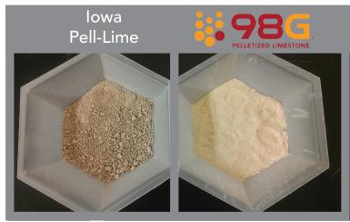
Particle size of material used to create pellets in the Iowa pell-lime (left) and 98G (right). Notice the significantly larger particles in the Iowa pell-lime (left) which result in slower and poorer performance in the field.
